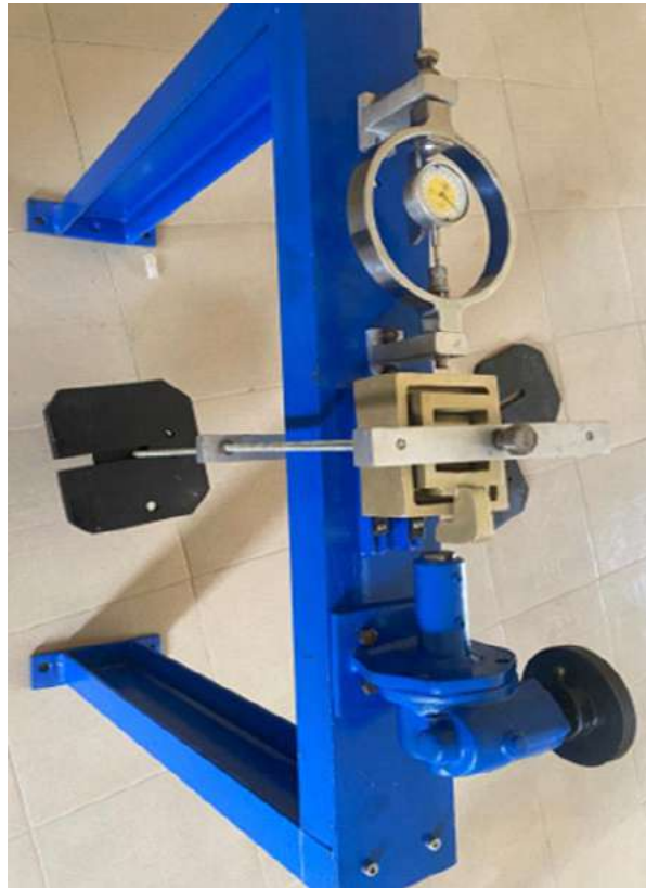
Plate 3: Assemblage of the Shear Box Machine (side view)
